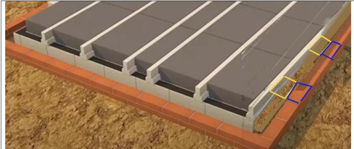
Right of the image depicts the dining area outside wall the blue rectangles are airbricks . The yellow rectangles need to be cut out of the filler of concrete so that air can circulate from the dining area through the airbricks into the cavity of the extension.
